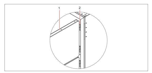
Fig. 7-1: Lift-off inner door
