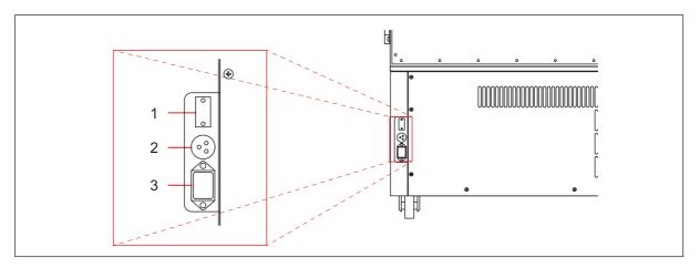
Fig. 6-3: Upright freezers alarm monitoring socket
