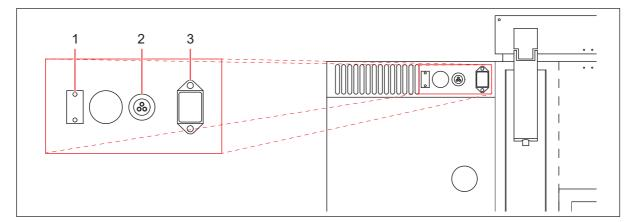
Fig. 6-4: Chest freezers alarm monitoring socket
