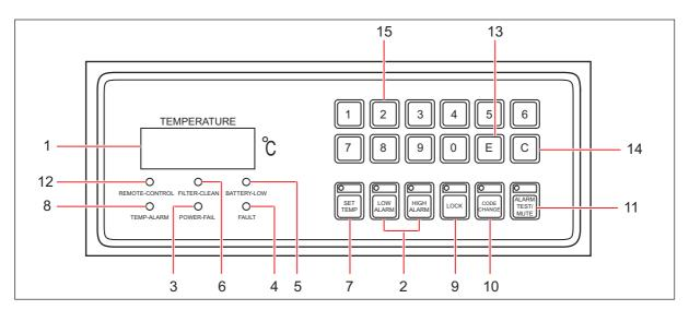
Fig. 5-1: Display panel & keypad
