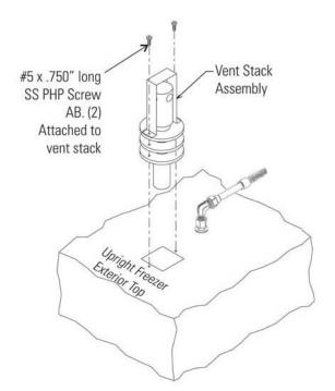
Figure 5-2. Vent Stack Assembly
