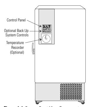
Figure 1-1. Freezer Front View Components
