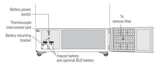
Figure 1-5. Battery(s) location and switch
