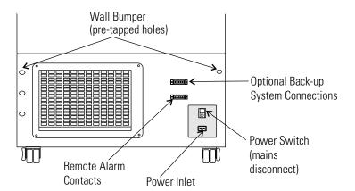
Figure 1-2. Freezer Rear View Components
