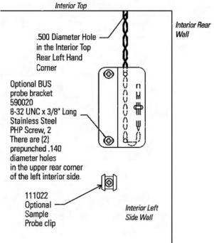
Figure 5-4. Mounted probe clip
