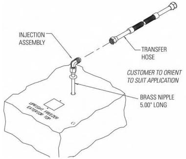
Figure 5-1. Injection Assembly
