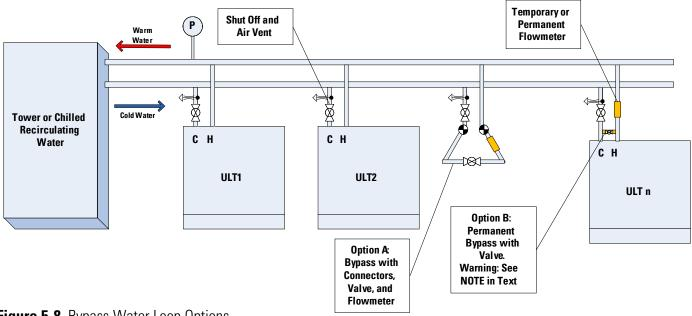
Figure 5-8. Bypass Water Loop Options
