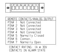
Figure 1-8. Remote Alarm Contacts
