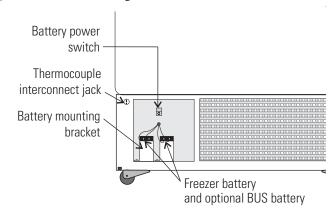
Figure 4-2. Battery Power Switch
