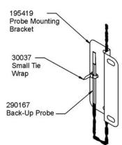
Figure 5-3. Secure probe
