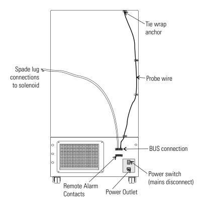
Figure 5-5. Probe wire and solenoid connections
