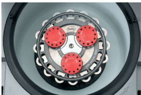
Figure 5: Retention plate in closed (secured) position. The curved lines on the retention plate align with the curved marks in the center on the shaft.
