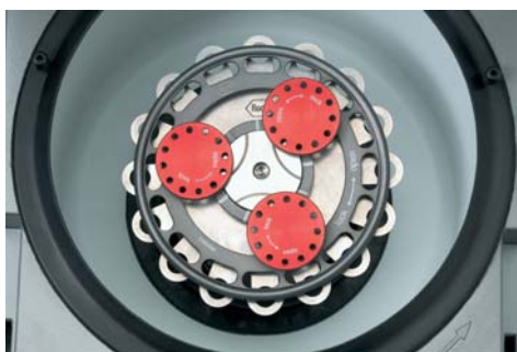
Figure 6: Retention plate in open (unsecured) position. The curved lines on the retention plate do not align with the curved marks in the center on the shaft.
