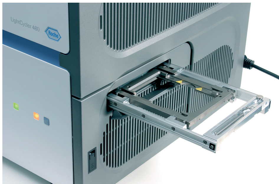
Figure 10 View of an ejected multiwell plate loader
