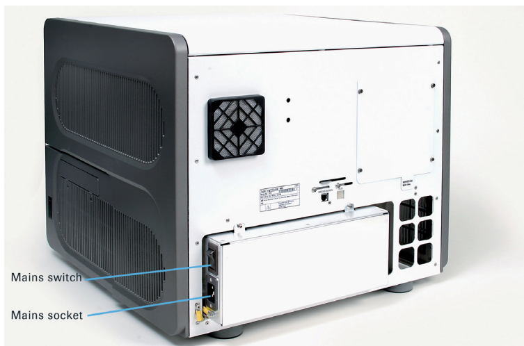
Figure 4 Location of mains switch and socket at the instrument's power box.
