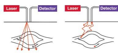
Laser Doppler emits light at a given frequency and then detects the frequency of the reflected light. Light that is reflected by moving particles, such as blood cells, experiences a frequency or Doppler shift which is proportional to the motion of the particle. That shift is used to determine the flow, velocity and mass of the blood.
